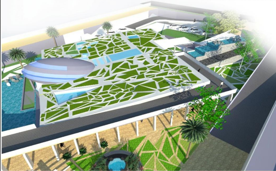
GREEN ROOF AND RAIN WATER HARVESTING IS PARTIALLY PROVIDED TO MAKE MUSEUM BUILDING AS ECO FRIENDLY BUILDING.
