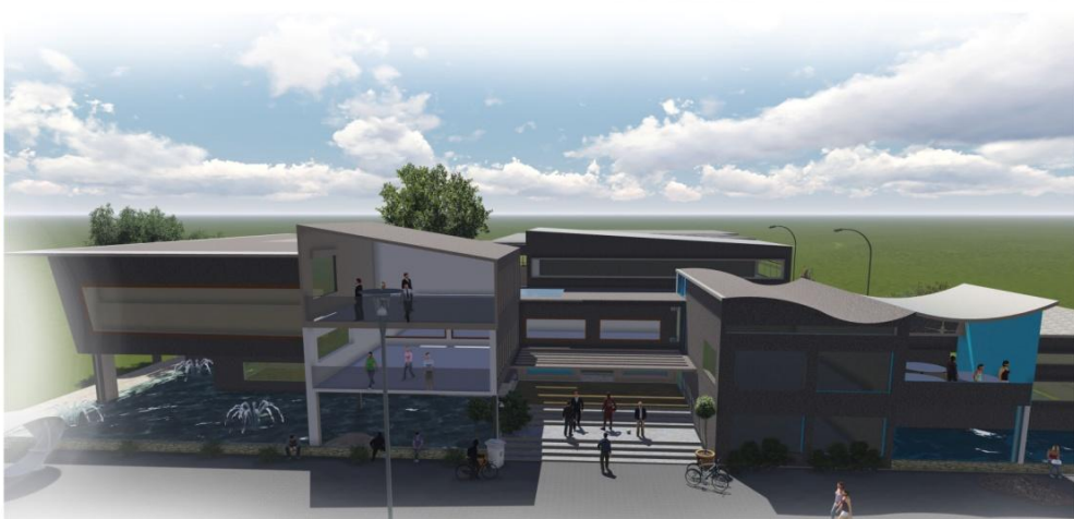
FRONT VIEW OF ARCHITECTURAL BLOCK SHOWING CANTILVERED DISCUSSION SPACE AND WATER BODY AS COOLING ELEMENT OF THE BLOCK
